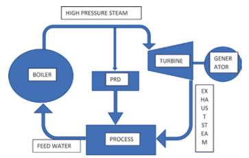
Figure 2 – Typical steam flow cycle in process industries
